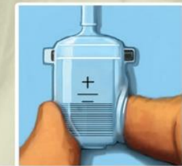
Pump Button to empty the Cuff after pressing and releasing it
