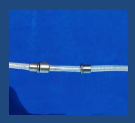
Connect the armed tubing with the connector.
